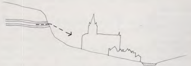
Drawing 1 Section through a typical valley, showing the steep escarpment between it and the plateau, the beds of grossier , and the usual relationship between the quarry and the nearby village church.
